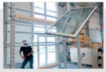
All our windows are drop tested, this tests the capability of the ironmongery to stop the window falling from the facade should any piece of ironmongery fail. VELFAC windows are proven to be safe and secure.
