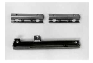
We salt spray test all exterior brackets after a Cyclic corrosion testing (evaluation value 10, EN/ISO 10289). The CCT test mimics the actual environmental impact in that the brackets are not only exposed to the salt spray, but also varying temperatures and alternating dry and humid environments. After the test (480 hours) all VELFAC brackets must still be without a trace of rust.
