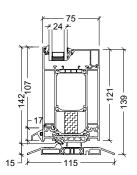
15mm ramped threshold with thermal break
