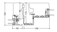
VELFAC 200 - VELFAC Ribo door Inward opening door Must be fitted with a cover profile.
