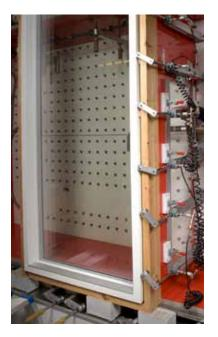
VELFAC 200 ENERGY casement door ready to open and close 20,000 cycles during an internal test at VELFAC, which is an integral part of the development process.
