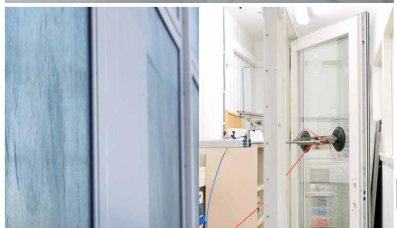
Top: Hose-test and Static water test at the 6.2m wide x 10m high CWCT test rig
