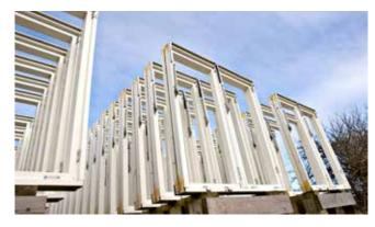
VELFAC frames exposed to high winds, rain and sun. This tests the durability of different surface treatments.
