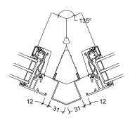
45° corner post, type A2202 45° aluminium pressing, type A1202
