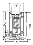
15mm ramped threshold with thermal break
