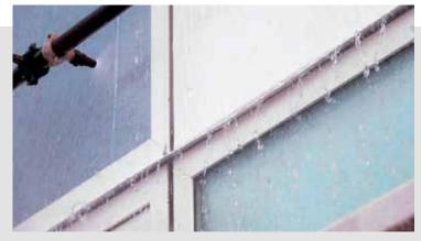
Window façade exposed to CWCT water load test. Water nozzles are located directly in front of the façade and water pumps with a flow rate of at least 3.4 litres/m²/minute.
