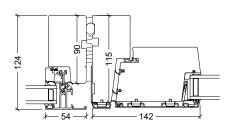
VELFAC 200 - VELFAC Ribo door Outward opening door Must be fitted with a cover profile.
