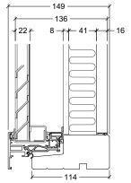
VELFAC 200 ENERGY louvre panel with intermediate board and backboard
