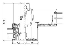
VELFAC 200 ENERGY - VELFAC Ribo Inward opening door Must be fitted with a cover profile.
