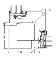
90° corner post, type A2002 90° aluminium pressing, type A1002
