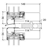
VELFAC 200 ENERGY - VELFAC 200 ENERGY Vertical coupling with drip flashing. Drip flashing is required for every 3 m min.
