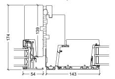
VELFAC 200 ENERGY - VELFAC Ribo Outward opening door Must be fitted with a cover profile.
