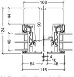
Mullion with uniform sightline window to the left and tophung fully reversible window with slightly different sightlines to the right
