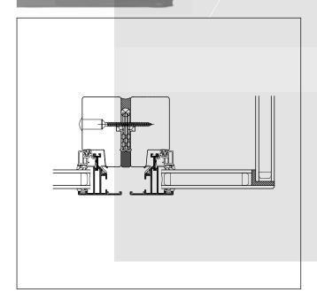
Corner window detail, structural fixing
