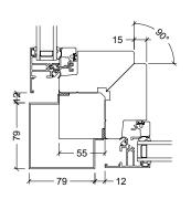
90° corner post, type A2001 90° aluminium pressing, type A1001
