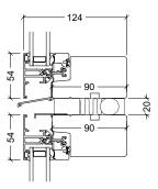
VELFAC 200 - VELFAC 200 Vertical coupling with drip flashing. Drip flashing is required for every 3 m min.
