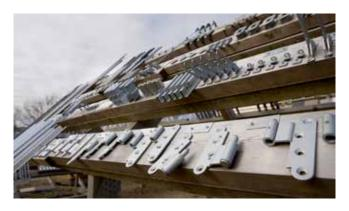
Our R&D Department develops the majority of VELFAC ironmongery to ensure it is ideally suited to the style and function of the VELFAC system, and all items are regularly tested both by VELFAC and by independent testing bodies. Here, VELFAC ironmongery is exposed to salt-laden winds and coastal weather conditions.
